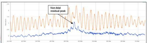
Major flooding in the Tweed River occurred in March 2022. Water levels measured at the water intake jetty (figure bottom left) show a non-tidal residual of over 1m at the peak of the flood.
